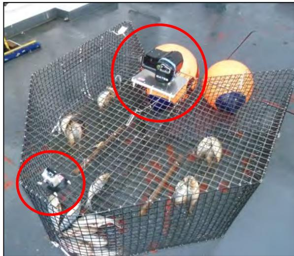
**Figure 6.1.** Chevron trap fully baited and rigged. The cameras (circled in red) are shown in one of several configurations used; in this one, they were located at the nose and the mouth of the trap. Photo: MARMAP/SCDNR
