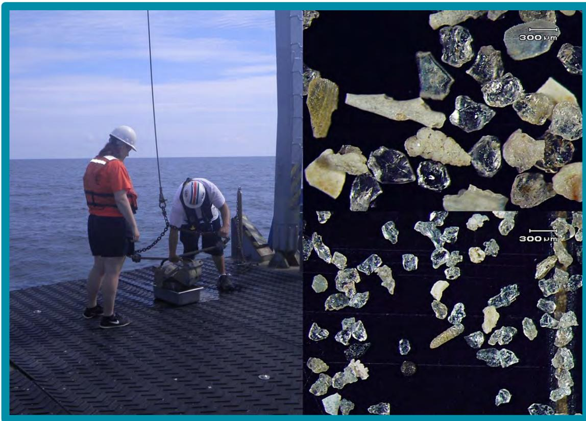
Left: Researchers collect seafloor sediments using a Van Veen Grab Sampler. Right: Clear quartz grains dominate sediments from the Georgia shelf, but biological components are also commonly observed. Photos: Claudia Venherm/UGA Skidaway Institute of Oceanography
