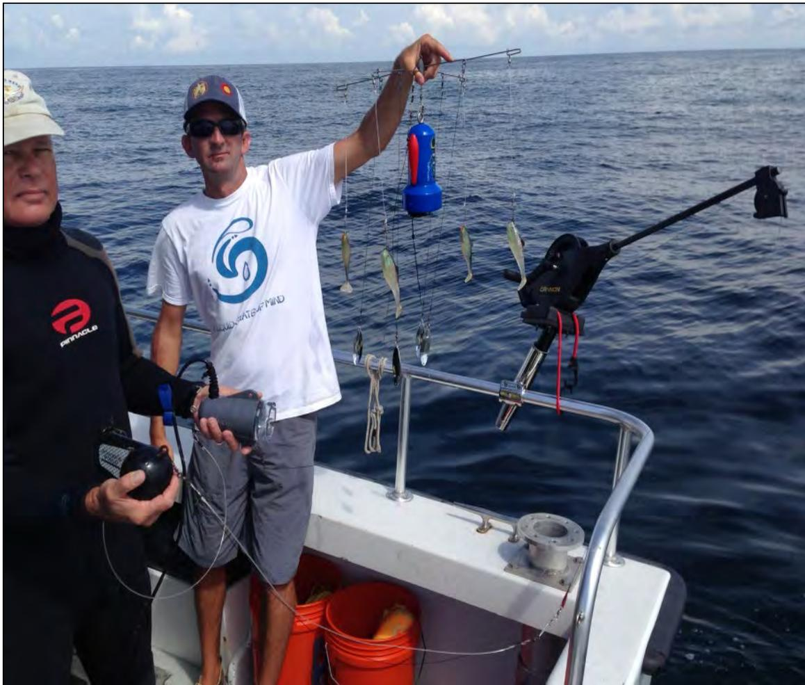
**Figure 12.2.** The Troll Pro (blue tow body) is arranged with a spreader in the center with artificial baits and spoons. The person at left holds the cannonball weight and SeaView drop camera. The drop camera, Troll Pro, and baits are lowered and towed from the downrigger at right. Photo: Peter Auster/University of Connecticut/Mystic Aquarium
