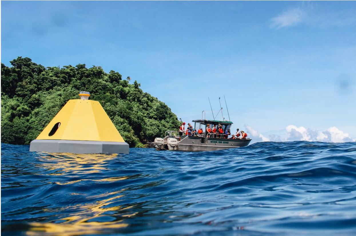
Monitoring environmental variables that can inform us about climate change using technology like this Ocean Acidification Buoy in the National Marine Sanctuary of American Samoa, deployed by NOAA's Ocean Acidification Program is an important way ONMS can track and understand climate change.
