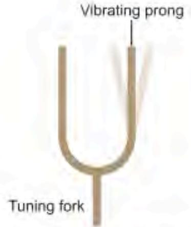
Sound produced by vibrating prong of tuning fork.
