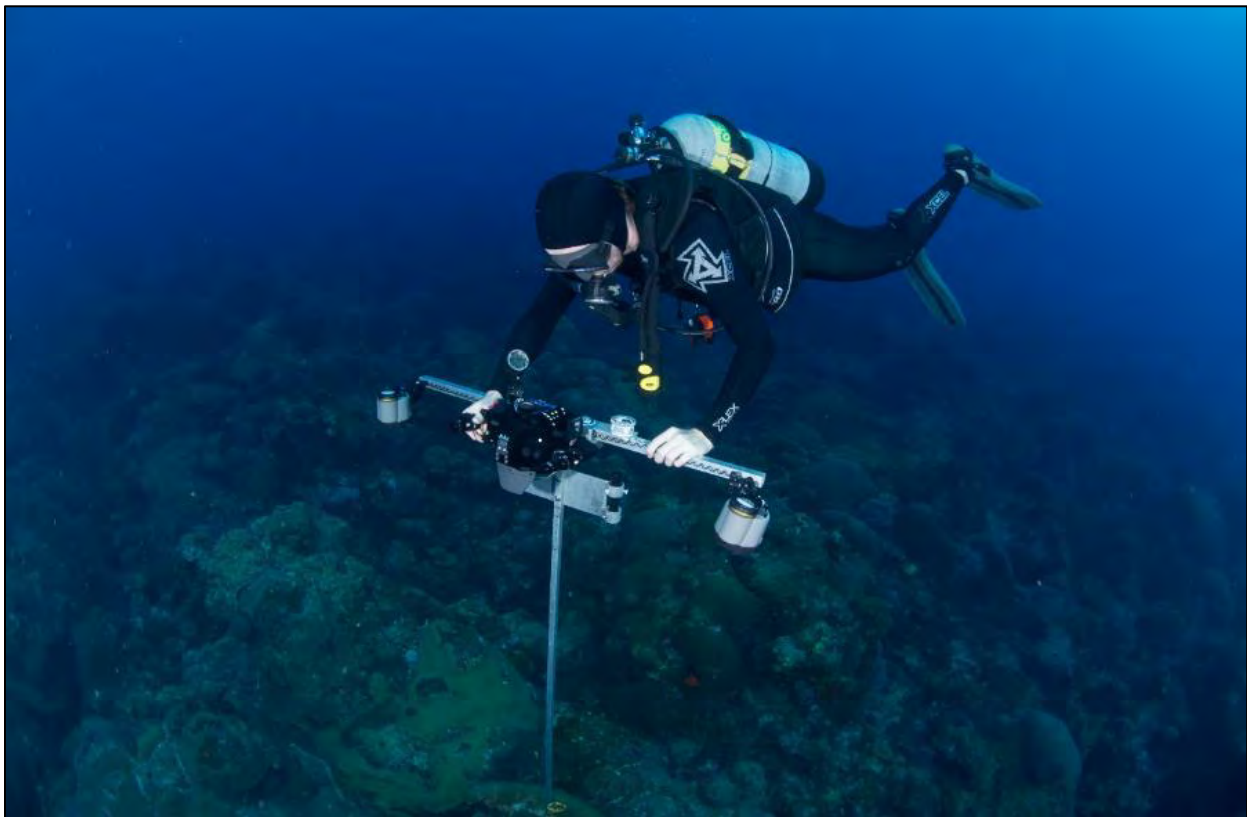
Figure 2.1. A NOAA diver photographs a repetitive photostation using a camera and strobes mounted to an aluminum T-frame. Photo: G.P. Schmahl/NOAA
