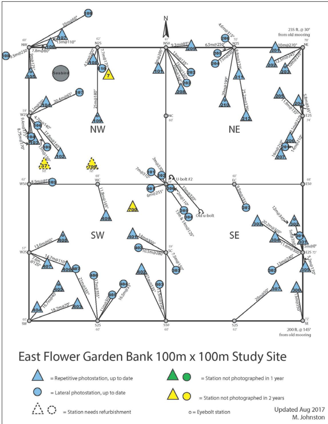
**Figure 1.5.** Detailed map of the EFGB study site and photostations in 2017. Permanent study site corner markers and eye-bolts installed at 25 m intervals along each perimeter and crosshair line. Reference lines are used to mark the north-south and east-west crosshairs. Establishment of the perimeter and crosshairs divide each site into four 50 m x 50 m quadrants.
