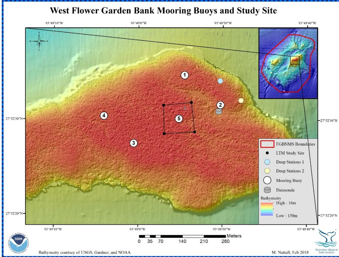
Figure 1.4. Bathymetric map of WFGB with long-term monitoring (LTM) study site, mooring buoy, water quality datasonde, and repetitive deep photostation locations.
