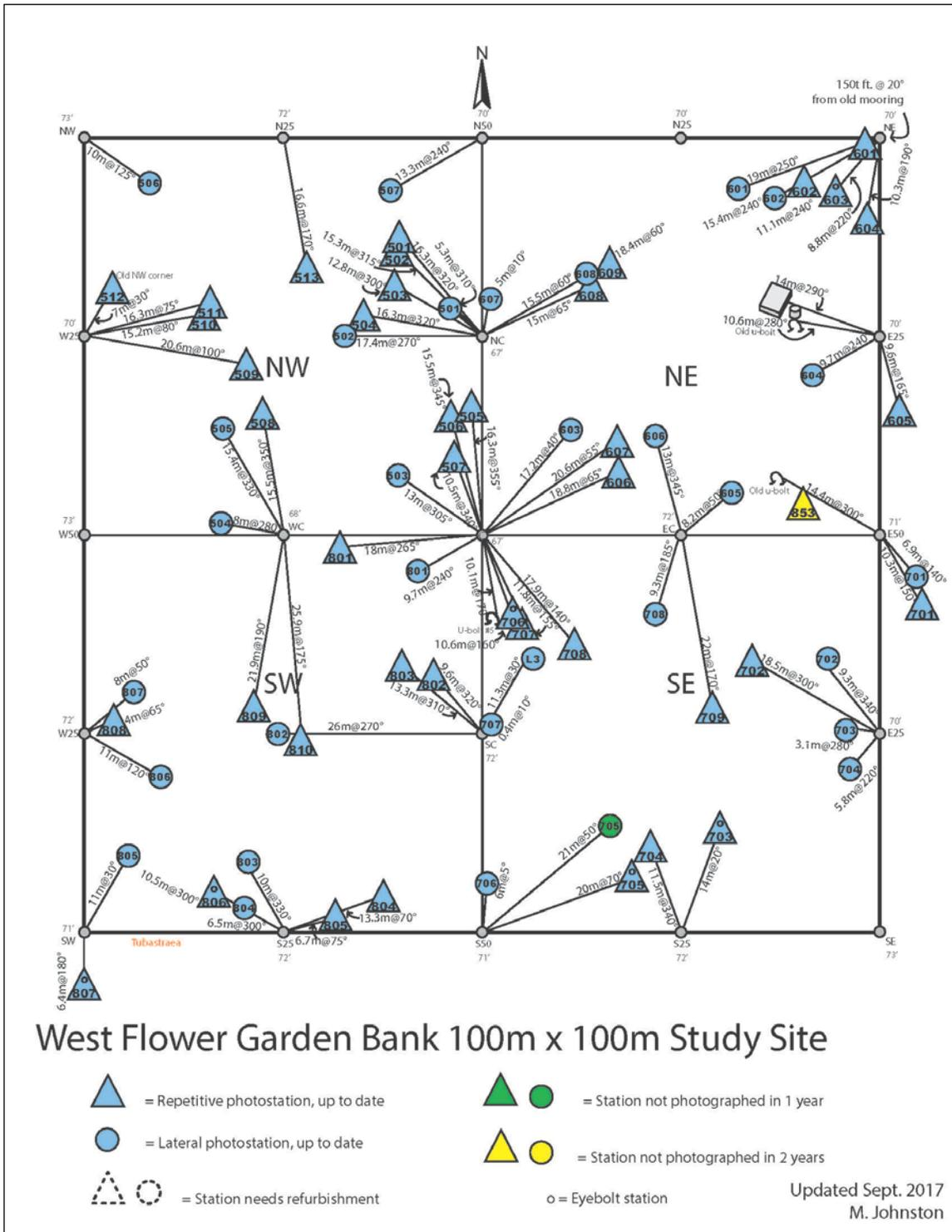
**Figure 1.6.** Detailed map of the WFGB study site and photostations in 2017. Permanent study site corner markers and eye-bolts installed at 25 m intervals along each perimeter and crosshair line. Reference lines are used to mark the north-south and east-west crosshairs. Establishment of the perimeter and crosshairs divide each site into four 50 m x 50 m quadrants.
