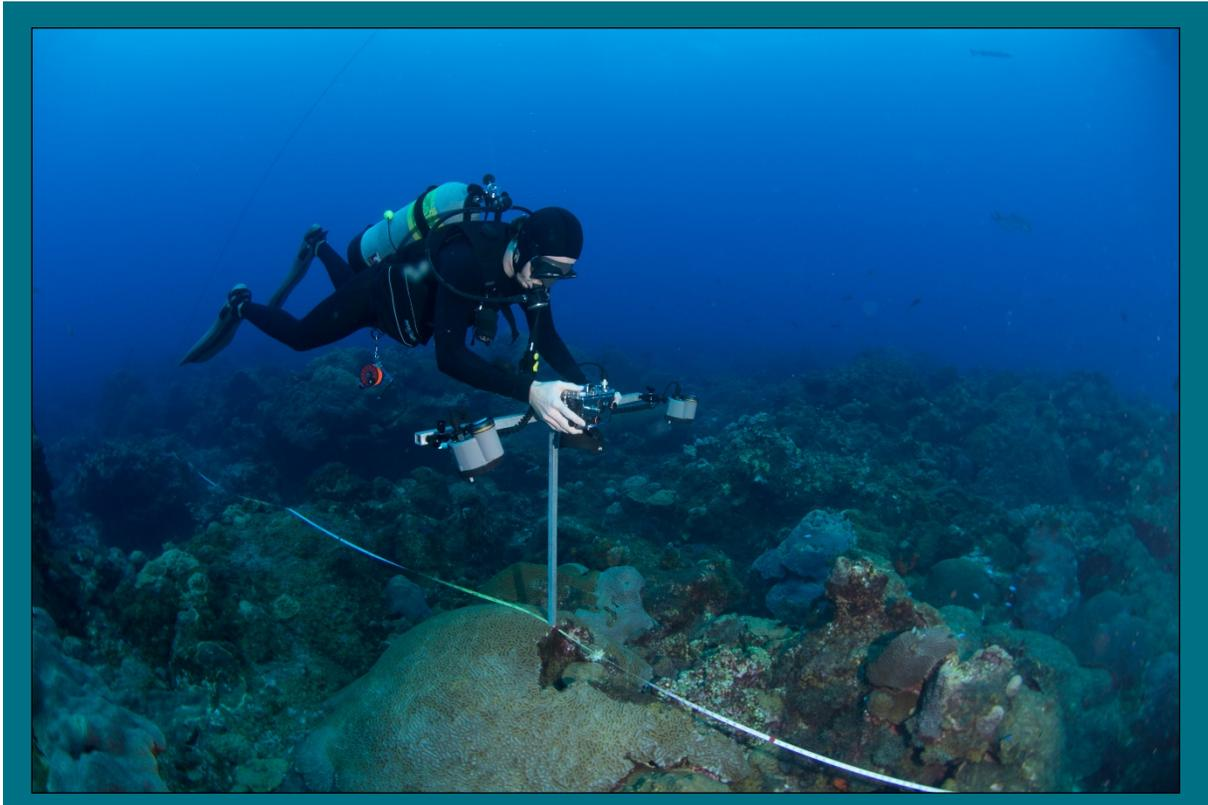
NOAA diver with camera and strobes mounted on an aluminum t-frame takes random transect photographs within the EFGB study site. (Photo: G.P. Schmahl, NOAA/FGBNMS)
