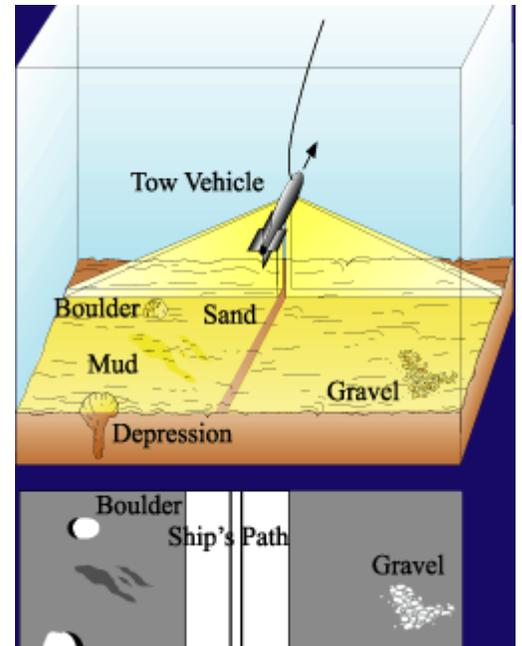
Side scan sonar diagram depicting the sonar pulses projecting from its transducers as well as the nadir under the towfish.
