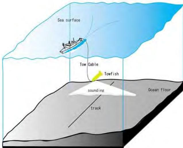
Research Vessel Towing the Side Scan Sonar Towfish
