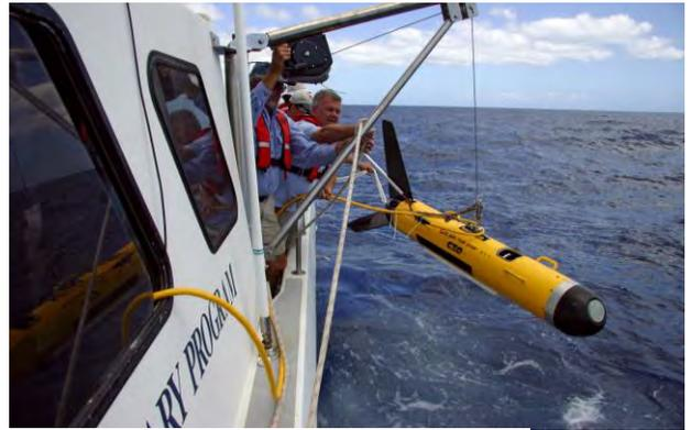
Side scan sonar towfish deployed off Hawaii (NOAA).
