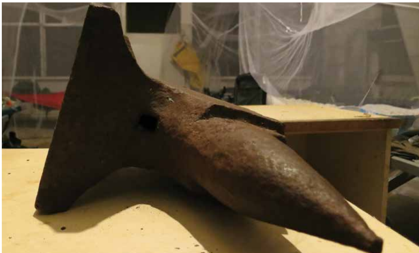
Figure 208: Front of anvil, showing handling hole
