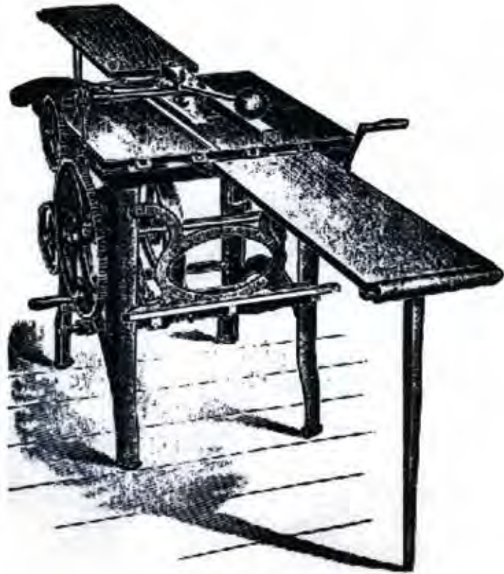
Figure 214: Catalog drawing of the Barnes Company table saw.
