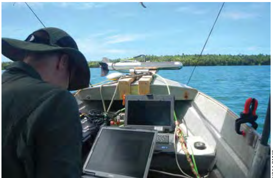
Figure 30: Tow fish ready for deployment and monitors on the skiff.
