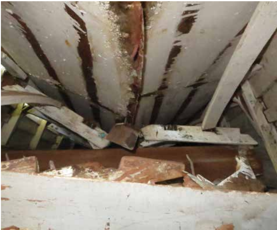
Figure 156: Interior view of the broken boat, cracked frames and floors.
