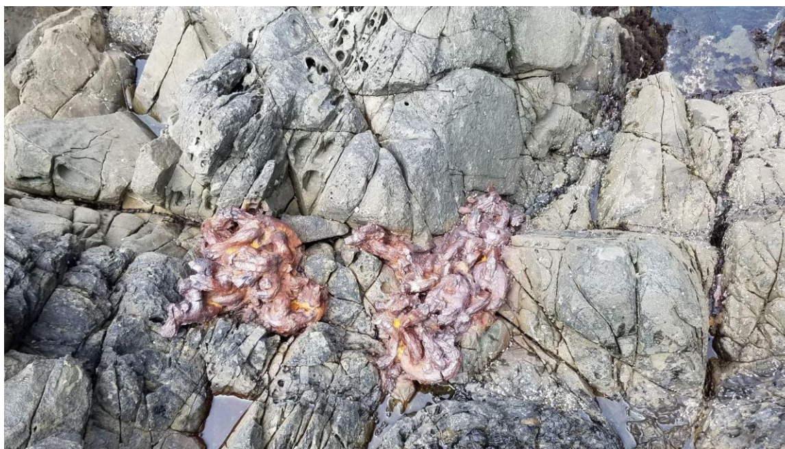
Figure S.MHR.16.5. Mooring hardware; a section of stud link chain pile at a doghole port site within the sanctuary. Photo: NOAA and California Department of Parks and Recreation
