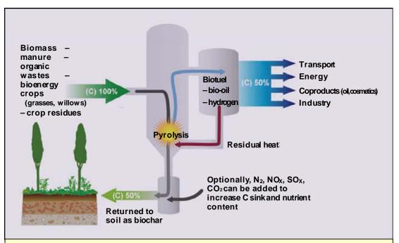
Figure 2: Concept of low-temperature pyrolysis bio-energy with biochar sequestration. Typically, about 50% of the pyrolyzed biomass is converted into biochar and can be returned to soil.
