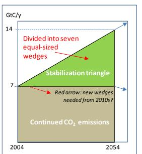
Figure 1 shows the basic Socolow/Pacala model. The stabilization triangle limits  $CO_2$  emissions to present levels. Each of seven technology "wedges" increases linearly until in 50 years it accounts for 1 GtC annually of reduced emissions. The seven-wedge assumption is based on a stabilization level of 500 ppm  $CO_2$  and emissions growing by 1.5%/year.
