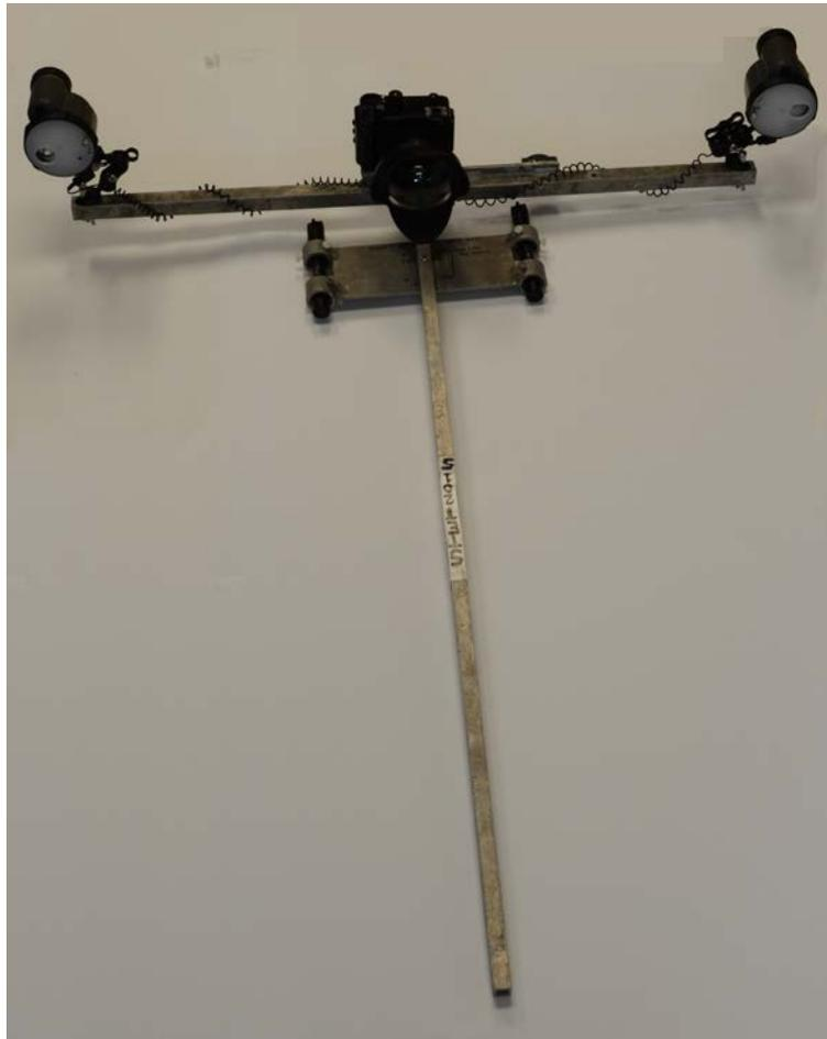
**Figure 1.4. T-frame configuration. G11 Fisheye FIX® housing mounted to the frame, set at 1.5 m from the substrate, with two Inon® Z240 strobes, set 1.2 m apart.**
