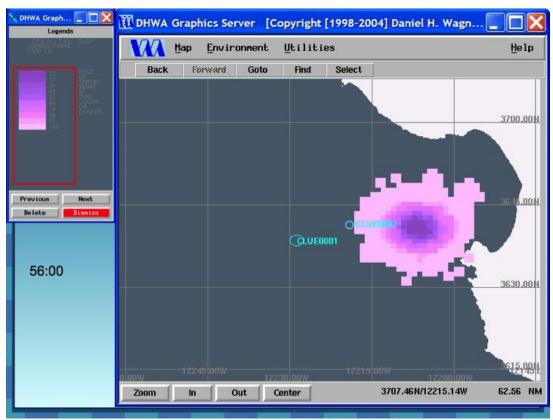
Figure 12. Modeling of likely drift of M/V *Med Taipei* containers after 56 hours. Clue0001 shows location of the container loss incident; Clue0002 shows the location of discovered container TGHU7712262. The darker the shade of purple, the greater the probability of containers being found within that area. Credit: Fugro Inc.
