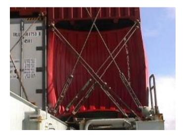
Figure 7. Lashing rods tightened by turnbuckles are attached by hand by longshoremen to help secure loads. (This container was damaged by a bow-slamming wave). Figure from Koning 2009.
