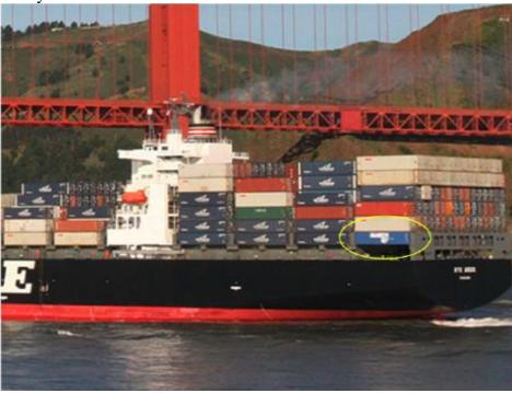
Figure 19. The *NYK Argus* leaving San Francisco Bay, with an instrumented MARIN container on the bottom tier to help monitor forces while underway. Photo credit: MARIN 2009.
