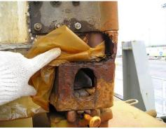
Figure 8. Container corner posts and fittings in unsatisfactory condition. Figures from AIMU 2008.
