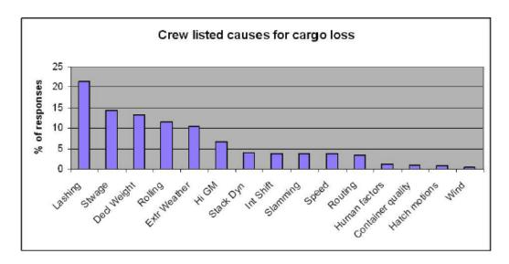
Figure 11. Crew listed causes for cargo loss. Factors named in order of frequency included lashing problems, poor weight distribution during stowage, inaccurate declared container weights, rolling, extreme weather, conditions leading to high metacentric height (GM), stack dynamics, internal cargo shifting, bow slamming, vessel speed, vessel routing, other human factors, poor container quality, hatch motions, and the effects of high winds. Figure from MARIN 2009.
