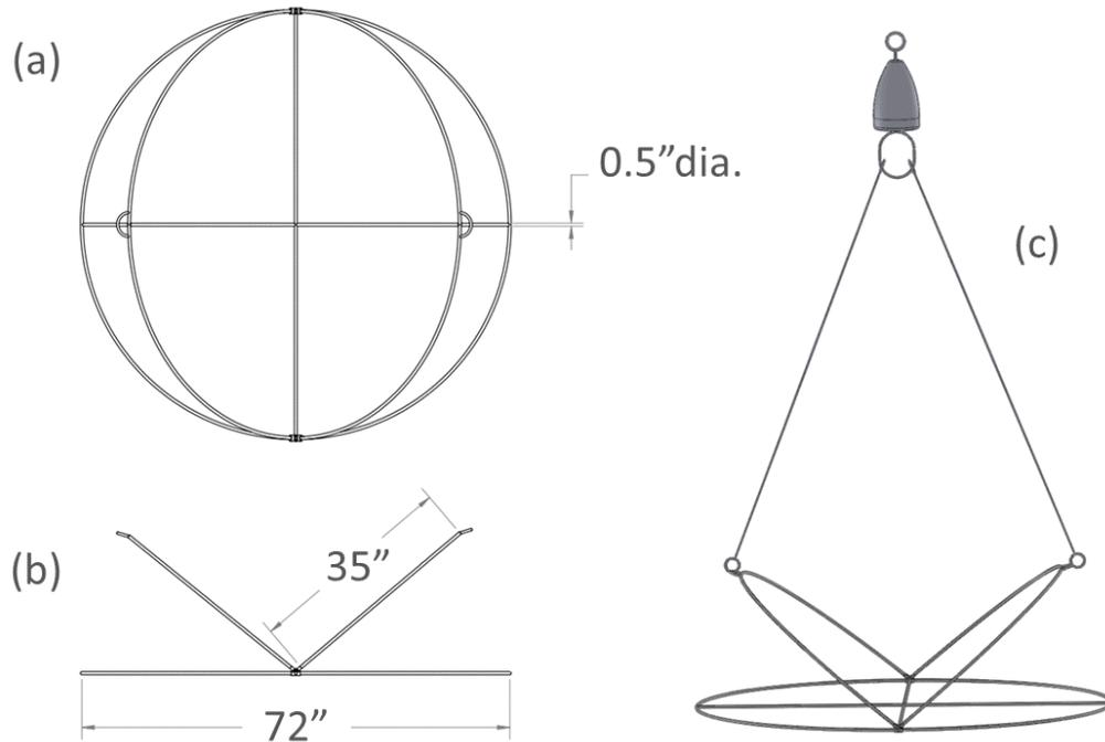
**Figure 3.** Shop drawings of Dome Trap. (a) top view of partially closed frame, showing one option for lift rings; (b) side view showing base (horizontal) and jaws (angled upward); (c) oblique view, showing another option for lift rings (as in Figure 4 below), and the two-line harness and float attached to the lift rings. (Image: Lewis Fortner, University of Georgia)
