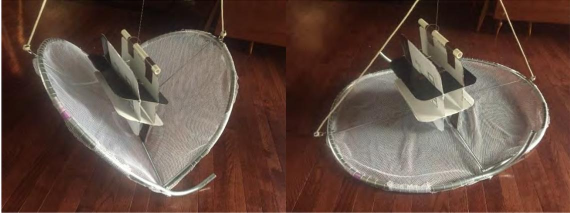
**Figure 8.** Mock-up Purse Trap and collapsible FAD partially open (left) and fully open (right). Note that the mesh covering this frame is tighter than it should be on an operating trap. A looser net would reduce the likelihood that the closing jaws would agitate fish. (Photo: Steve Gittings, NOAA)
