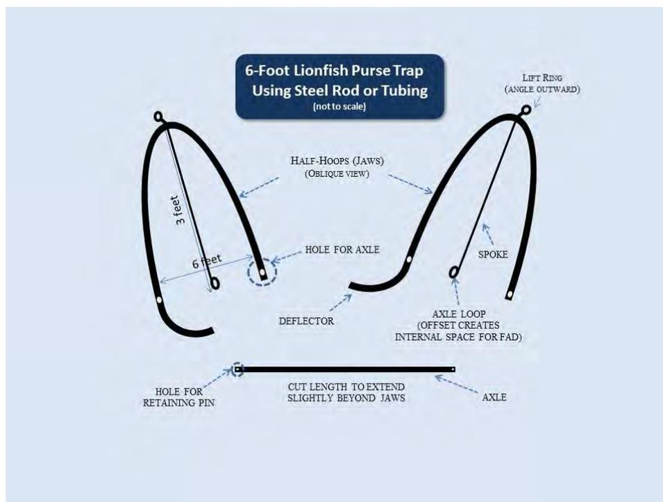
**Figure 7.** Oblique view of components of a 6-foot Purse Trap design for capturing lionfish. The jaws are two half-hoops, each with a curved extension on one end. The axle feeds through holes on the end of each hoop and the axle loop on the end of each spoke. When assembled, the curved extensions need to be outside the adjacent half-hoop. Lift rings angling away from each other allow the harness to force the jaws closed. (Image: NOAA)
