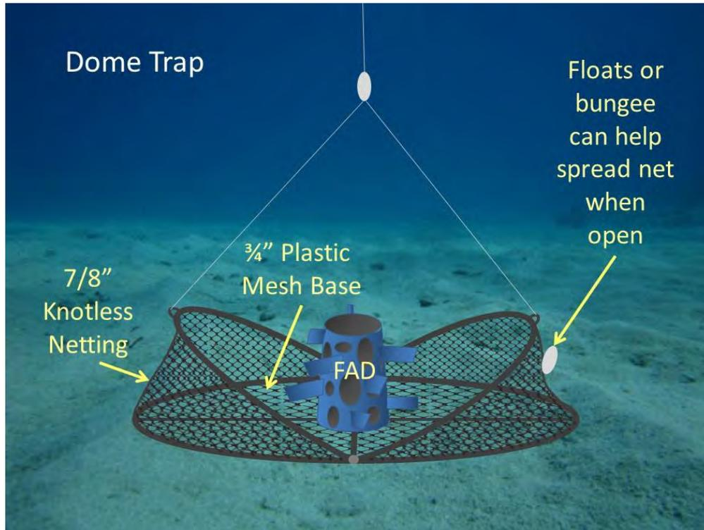
**Figure 2.** Diagram of partially closed Dome Trap. Small floats were attached to the net during initial tests to keep it away from the FAD when open. (Image: NOAA)
