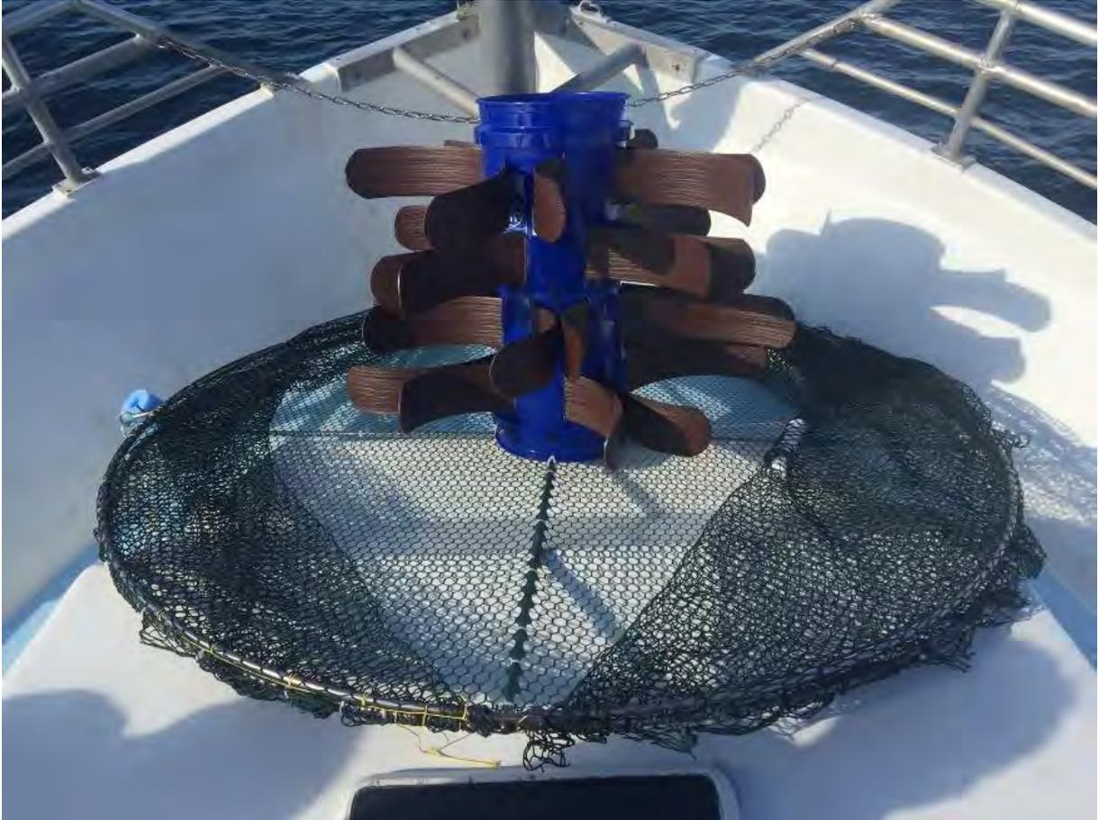
**Figure 5.** Trap frame complete with FAD (connected to crossbars) and attached net. Total weight of this frame is approximately 40 pounds in air, and it descends at a rate of about 80 feet per minute. (Photo: Steve Gittings, NOAA)
