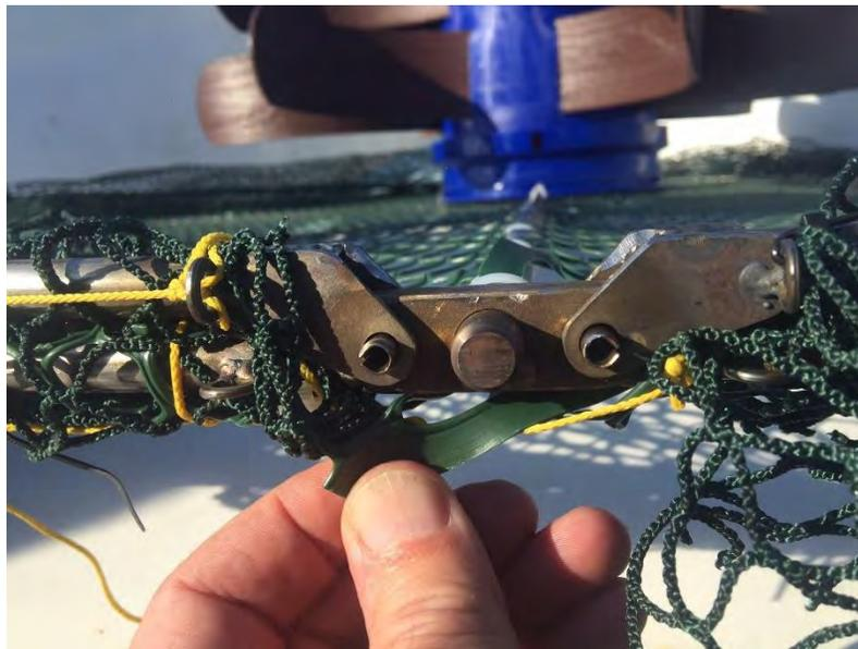
**Figure 4.** Configuration of dual hinge and spring pins holding jaws at end of central crossbar of trap frame. (Photo: Steve Gittings, NOAA)
