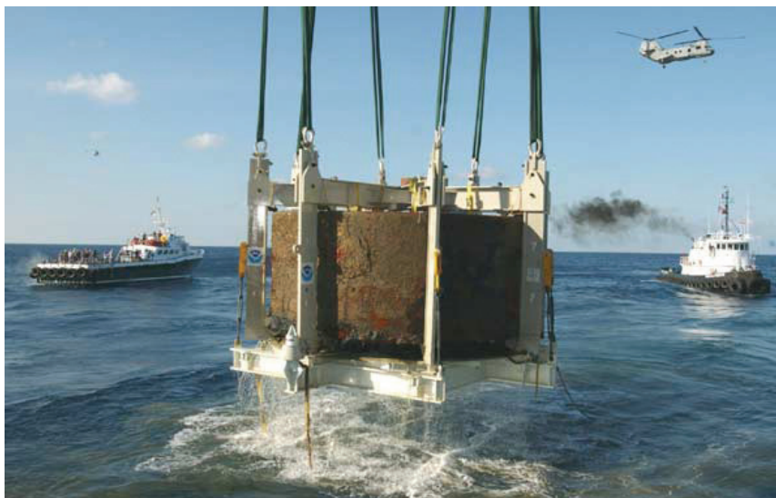
The Monitor 's steam-powered turret is a national icon that was the model for all turreted warships through modern times. The partnership that included NOAA and the U.S. Navy resulted in the recovery of the turret in 2002.
