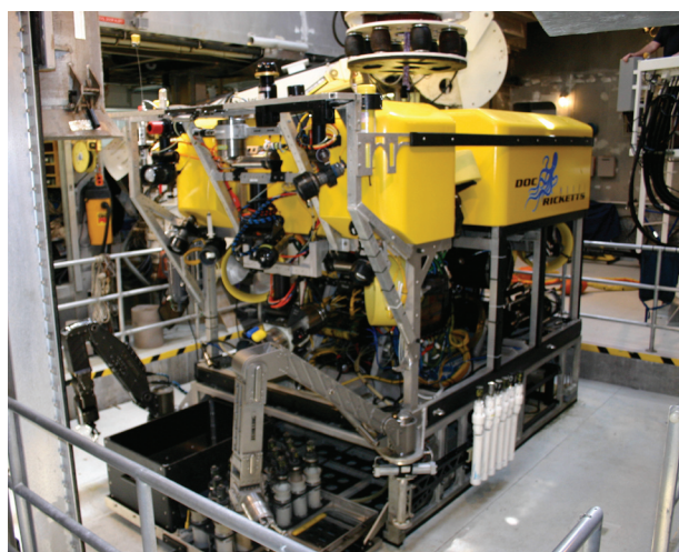
Figure 10. The ROV Doc Ricketts is a remotely operated vehicle used to explore the midwater and deep-sea habitats in the Monterey Bay region and broader Eastern Pacific ocean.
