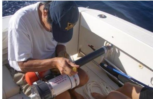
*Example of passive acoustic recording device (EAR).
