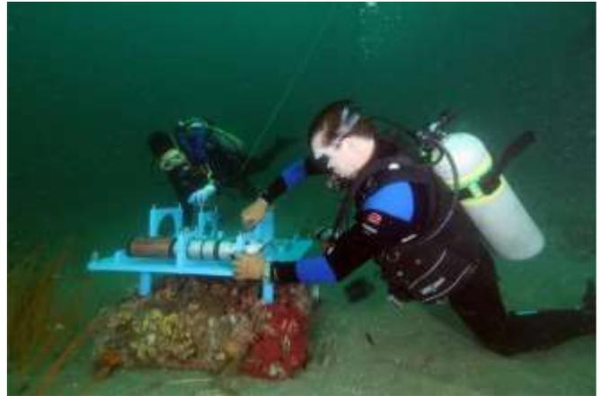
NOAA divers install the seafloor observatory that collects continuous  $p\text{CO}_2$ , pH, and temperature data. Photo Credit NOAA
