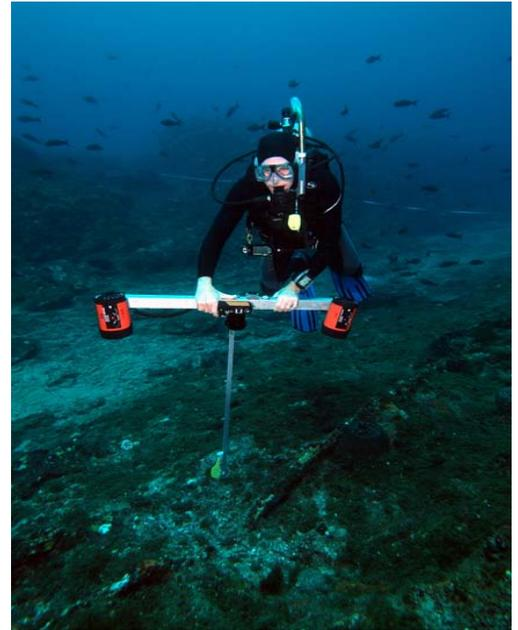
*Diver using T-frame camera system at Stetson Bank to collect repetitive photostation image for annual analysis. Photo credit: Joyce and Frank Burek.*
