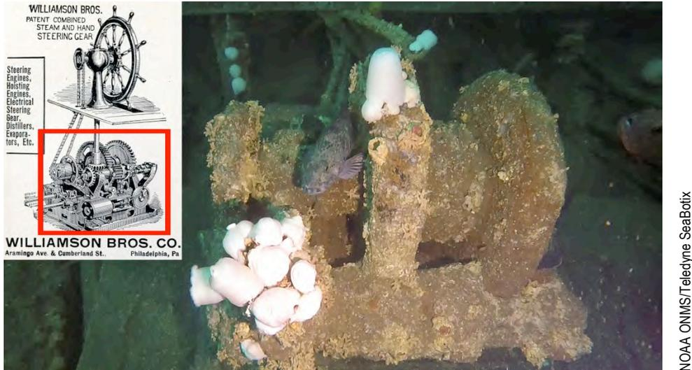
Fig. 7: Williamson Brothers patent combined steam and hand steering gear, lying inside the forward hull next to the 3-inch/50 caliber gun.
