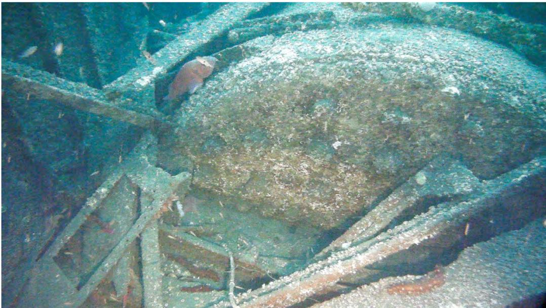
Fig. 8: Inside the boiler compartment, showing part of one boiler and collapsed debris from the upper works of the tug
