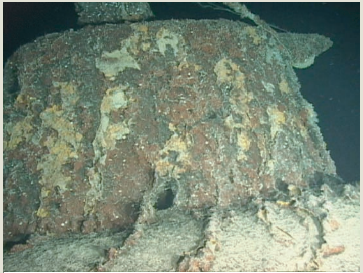
The conning tower of the Japanese mini-submarine, showing the 4-inch hole where the USS Ward hit and sank the vessel. This was the first shot between the U.S. and Japan in WWII.
