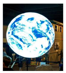
Science on a Sphere is a room sized, global display system that uses computers and video projectors to display planetary data onto a six foot diameter sphere, analogous to a giant animated globe. (Source: TBNMS)
