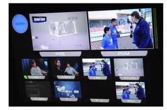
Multiple video monitor screens on a mobile telepresence unit showing both the underwater and presentation feeds. Telepresence is an innovative tool that can bring sanctuary research to the public. (Source: immersionlearning.org)
