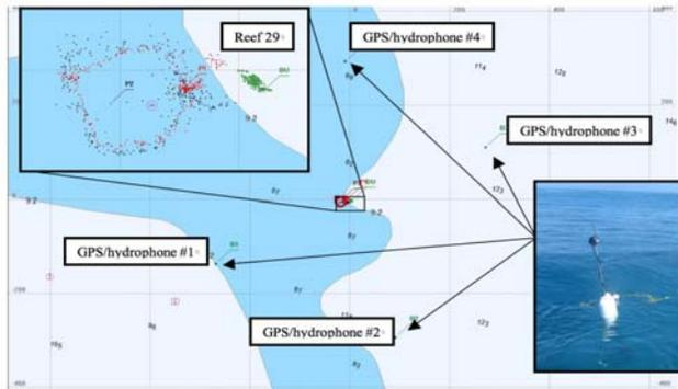
**Figure 3.** Map of GPS / hydrophone array positioned around Reef 29, a patch reef in French Frigate Shoals.
