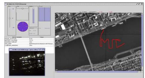
**Figure 23.** Schematic of the wireless AUV concept and interactive web-based interface (by Victor Polidoro, MIT AUV Lab).
