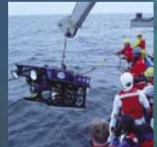
A ROV is lowered over the side of the R/V *Connecticut* during a survey of the wreck of the steamship *Portland*.
