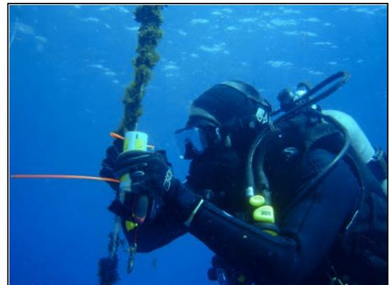
CINMS working diver, Julie Bursek, attaches a temperature logger to a subsurface mooring during biannual servicing of West Coast Obs Moorings. Photo credit: Claire Fackler, NOAA/ONMS.
