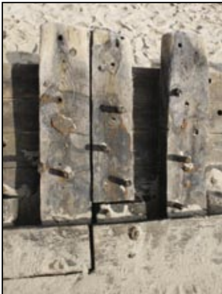
Trunnels (treenails) and trunnel wedges protrude from the massive frames.
